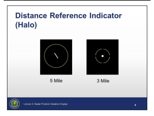
A five mile Distance Reference Indicator, also known as a halo, can be displayed around the aircraft target symbol to help maintain proper aircraft separation
