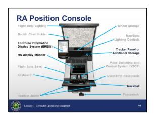
The RA Position Console has four components that are different from the A Position Console:
